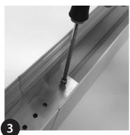
Pull the Suspension Wire tight after assembly to make sure joining bar is secure and tighten 4x screws.
