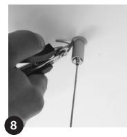
Cut the Suspension Wire to the desired Wire length.
